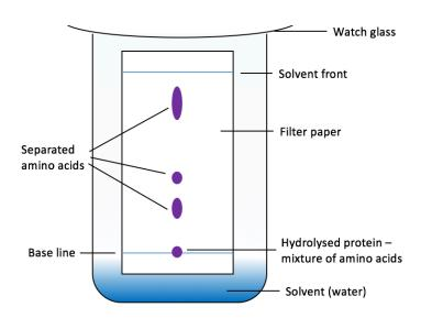
R<sub>f</sub> = <u>Distance moved by component</u> Distance moved by solvent front
